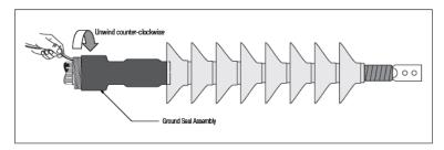
5. Shrink the Lug Seal Tube covering the top of the skirted assembly and onto the lug barrel.
