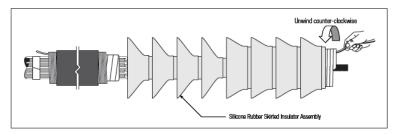
4. Shrink the Ground Seal Tube at the bottom of the termination.
