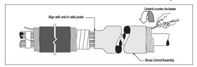
3. Install the Cold Shrink Silicone Rubber Skirted Assembly.
